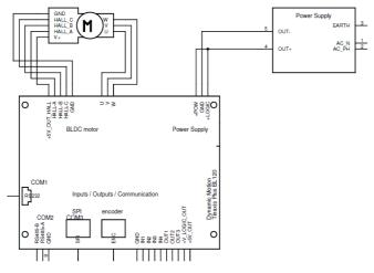
The following examples illustrates how to connects inputs. NEVER connect together GND from power side and I/O side, it already connected inside the board.
