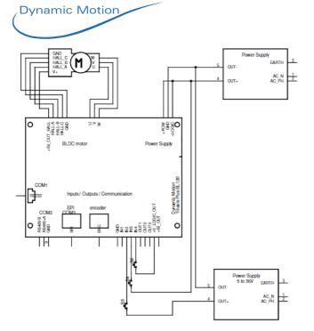
3 examples of wiring digital inputs: Using connection to the same power supply, separate power supply and 24V I/O connector output V\_Logic
