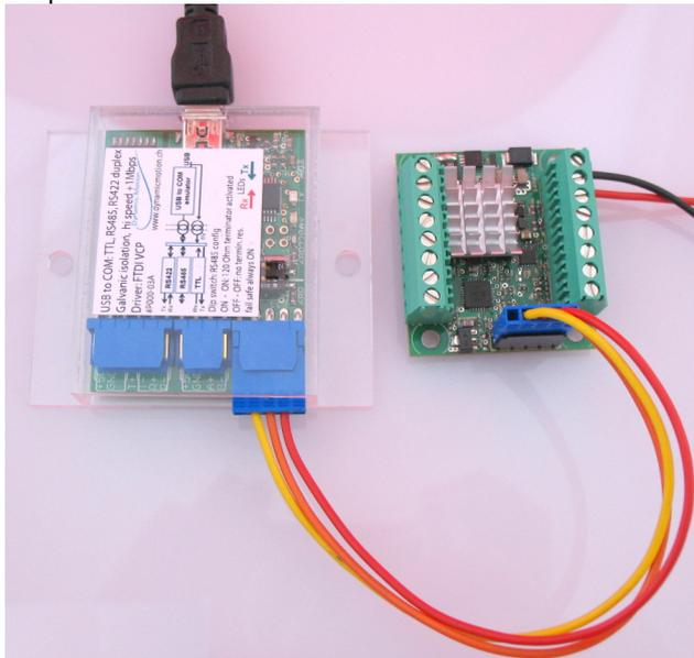
Figure 4: Supply the board with an external source and connect the interface
